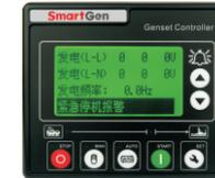
1. Control and protection for fuel gas engine and generator
