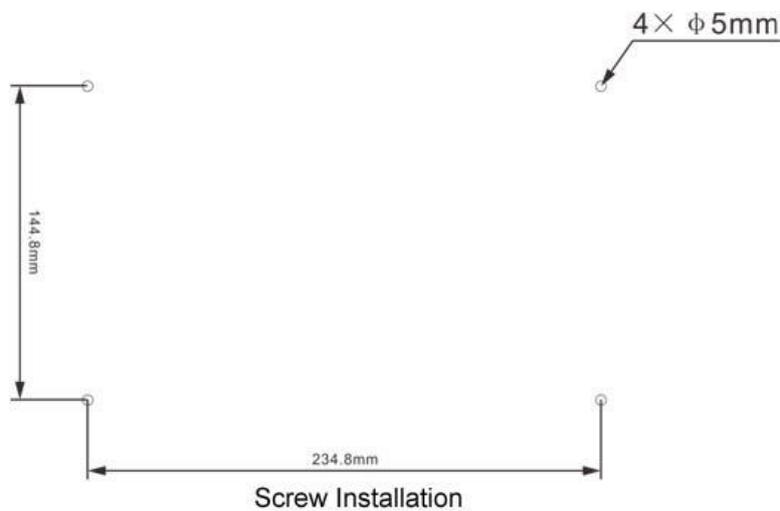
**Fig. 15 Screw Installation**
