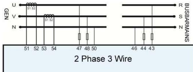
**Fig. 5 2-Phase 3-Wire Typical Application Diagram**
