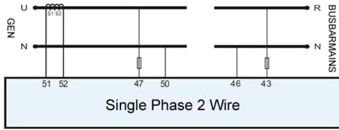
**Fig. 6 Single Phase 2-Wire Typical Application Diagram**
