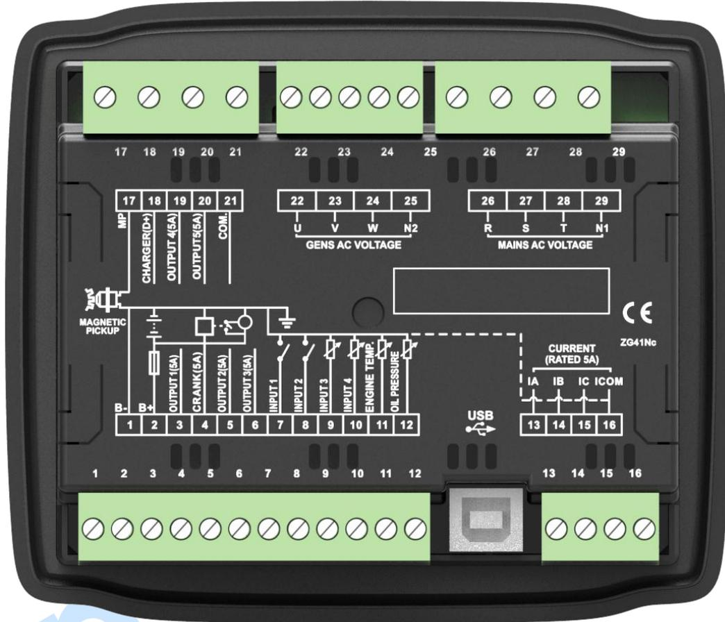
**Fig.2 Controller Rear Panel**
